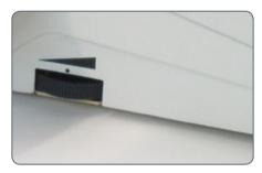
4. Turn on the microscope using the switch on the bottom right-hand side of the microscope stand.
